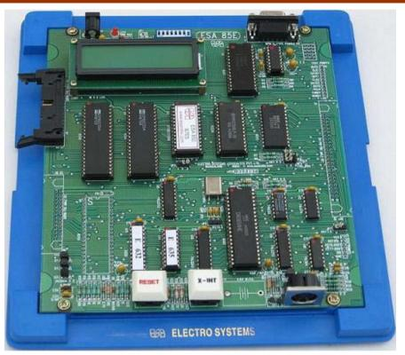
ESA 85E is the economy model of MPS 85-3 Microprocessor trainer based on the popular 8085 CPU with onboard LCD and PC connectivity through its RS-232-C port. ESA 85E can be used as a flexible instructional aid in academic institutions.
