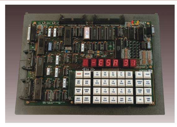
MCS-51 family of microcontrollers is increasingly becoming popular for instrumentation and control applications due to its speed and powerful instruction set which are essential for real-time applications. This has created the need for a good trainer and development tools. ESA 31 provides complete solution for this requirement. It can be used as a flexible instructional aid in academic institutions and a powerful development tool in R&D Labs.
