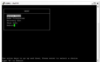
1. Update Image: this option can recover the loader, kernel and file system by using an USB disk. The USB disk contains the images files with the path as follow:
