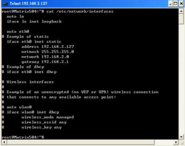
Use *vi* editing tool to edit the /*etc/network/interfaces* for network setting. The default setting is static IP 192.168.2.127. M-506 also supports Wireless LAN. Use
