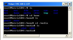
The 128MB NAND Flash memory of M-506 contains Boot loader (uBoot), Linux Kernel, Root File System and user disk (\home). The file system and disk space are shown as follow
